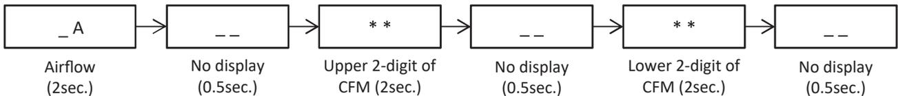
The contents indicated at 7 segment display vary according to operation mode and status of indoor unit. In the event of showing some error code, please follow the instruction in the table of indoor unit error code to solve the error.
