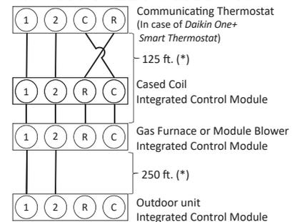
It is **strongly** recommended that you do not connect more than two wires into a single terminal in the field because there is a risk of the wires becoming loose, which may result in intermittent operation.
