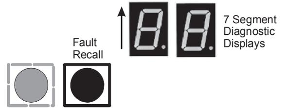
**NOTE:** For the cased coil application, the active error codes displayed on this control board are information related only to EEV cased coil.
