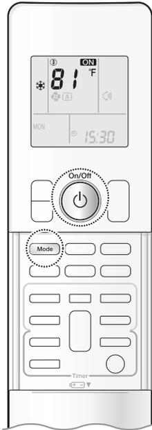
The air conditioner operates with the operation mode of your choice. From the next time on, the air conditioner will operate with the same operation mode.
