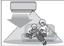
The air conditioner is in normal operation while the sensor is detecting human movement.
