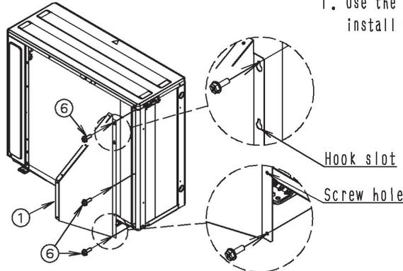
1. Use the 3 piercing screws ⑥ included in the kit to install the side plate (right) ①.
