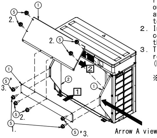
1. Align the bent surfaces on the left and right of the rear plate (4) with the outer surfaces of the side plate (left) (1) and side plate (right) (2), then tighten temporarily with 2 screws (5).
