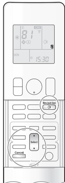
The CLEAN function dries the interior of the indoor unit to reduce the amount of condensation present. When COOL or DRY operation is performed, condensation may occur inside the air conditioner. It is recommended to dry the inside of the air conditioner using CLEAN operation.
