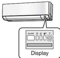
The wireless LAN connection adapter lamp blinks for 1 second.
