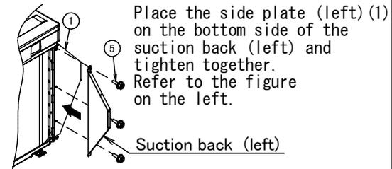
Place the side plate (left) (1) on the bottom side of the suction back (left) and tighten together. Refer to the figure on the left.
