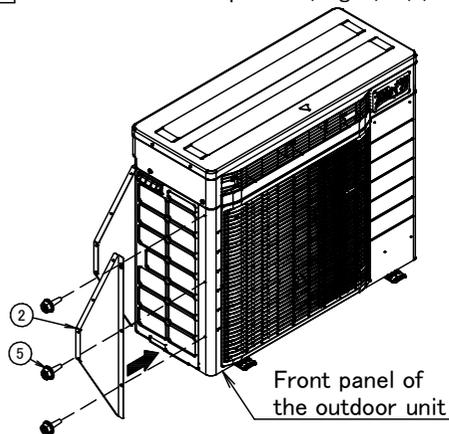
1. Install the side plate (right) (2) on the left side of the front panel of the outdoor unit using 3 screws (5).
