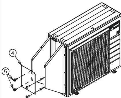
1. Temporarily secure the front plate ④ in place with the 4 screws ⑤.
