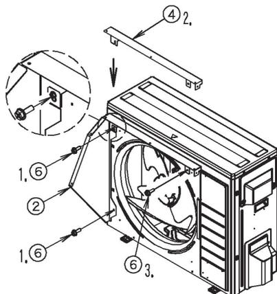
1. Temporarily secure the side plate (left) ② in place with the 2 piercing screw ⑥ included in the kit.
