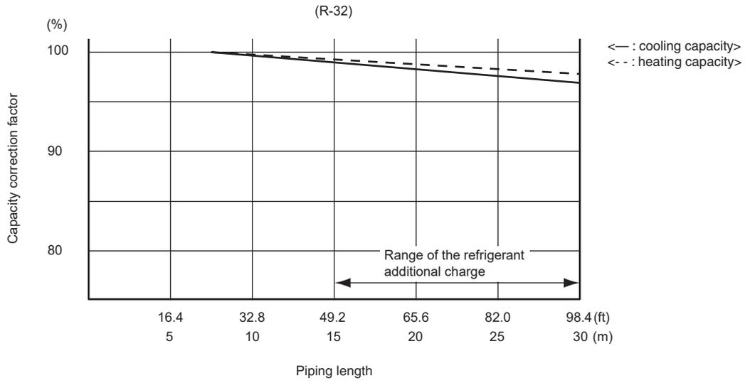
**Note:** The graphs show the factor when additional refrigerant of the proper quantity is charged.
