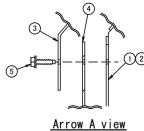
4. Securely tighten the 8 screws (5) that were temporarily tightened in steps 1, 2, and 3.
