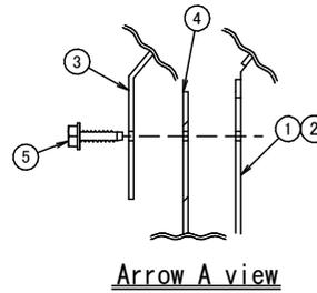
4. Securely tighten the 10 screws (5) that were temporarily tightened in steps 1, 2, and 3.
