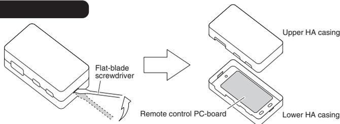
② Lift the handle of the screwdriver upward.
