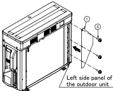
1. Install the side plate (left) (1) on the back of the left side panel of the outdoor unit using 3 screws (5).
