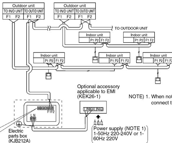
NOTE) 1. When not using the optional accessory applicable to EMI (KEK26-1), connect the power supply wiring directly to the unified ON/OFF controller.
