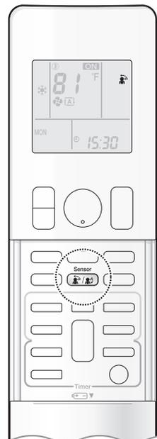
The INTELLIGENT EYE sensor detects human movement and adjusts airflow direction. It can be set to avoid people or to direct airflow specifically at people. If no one is in the room for more than 20 minutes, the operation automatically changes to energy saving operation.
