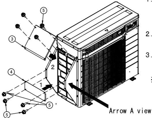
1. Align the bent surfaces on the left and right of the front plate (4) with the outer surfaces of the side plate (left) (1) and side plate (right) (2), then tighten temporarily with 2 screws (5).
