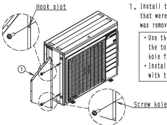
1. Install the side plate (right) ① with the 2 screws that were used in the protective wire mesh that was removed in step 1.
