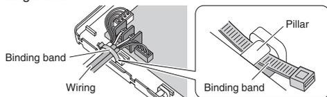
② Insert the second binding band into the groove on the side of the HA casing and fix the wiring securely so that the wiring will not be disconnected.
