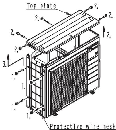
1. Remove the 2 screws that hold the protective wire mesh.
