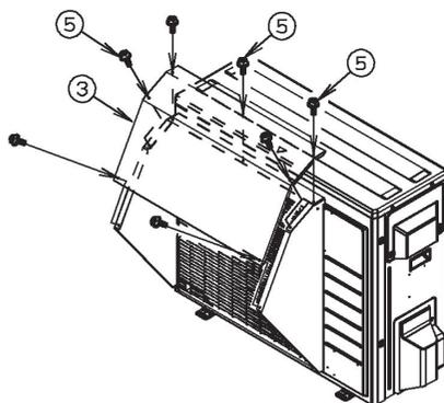
1. Install the top plate ③ with the 7 screws ⑤ included in the kit.
