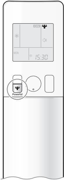
POWERFUL operation quickly maximizes the cooling (heating) effect in any operation mode. In this mode, the air conditioner operates at maximum capacity.
