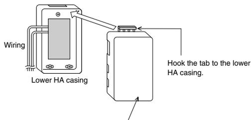
Press the lower part of the upper HA casing and press fit it onto the lower HA casing. Press the upper HA casing precisely until a clicking sound is heard.
