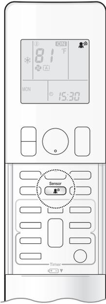
The INTELLIGENT EYE operation detects human movement. If no one is detected in the room for more than 20 minutes, the unit automatically enters energy saving operation.
