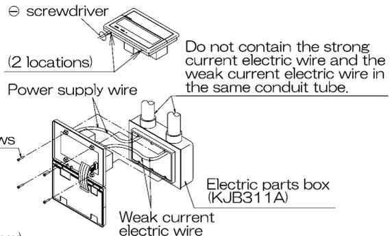
NOTE) Suitable length of the electric wire is about 160mm. (from electric parts box) If it is difficult to contain a long wiring, strip the sheathed part of the wiring.
