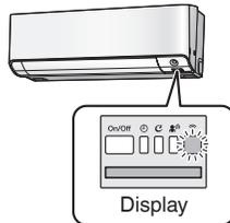
The wireless LAN connection adapter lamp blinks more quickly.
