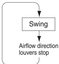
The horizontal airflow direction louvers move up and down.
