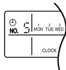
3. Press the **BUTTON FOR SELECTING DAYS OF A WEEK**, and set the proper day of the week. Each time you press it, the flashing display of days of a week shifts to the right.
