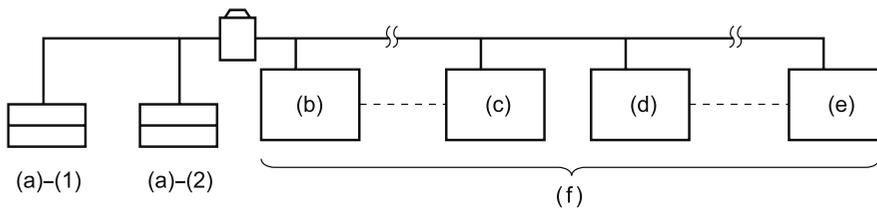
With two central remote controllers, centralized control (indoor units) is possible from different locations.
