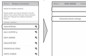
**8. Make sure that the wireless LAN connection adapter lamp has changed from blinking to lit. After it has changed, tap “On continuously”.**
