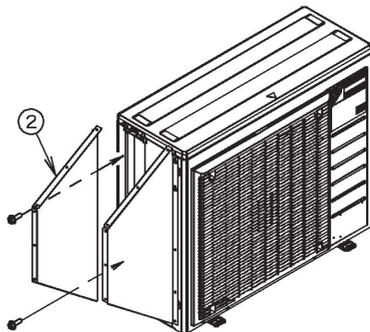
1. Install the side plate (left) ② with the 2 screws that were used in the protective wire mesh that was removed in step ①.
