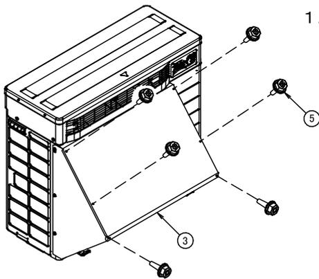
1. Install the top plate (3) on the side plate (left) (1) and side plate (right) (2) using 6 screws (4).
