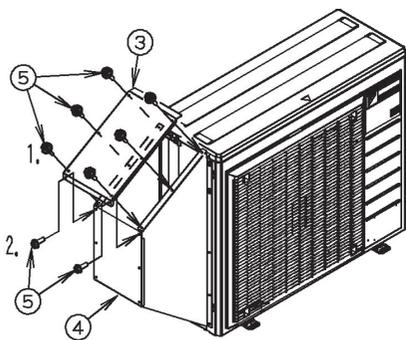
1. Attach the top plate ③ with the 6 screws ⑤.
