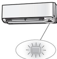
■ **Check the interval time between blinks of the OPERATION lamp.**
