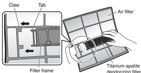
**3. Clean or replace the titanium apatite deodorizing filters.**
