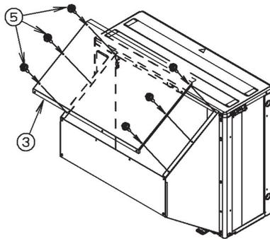
1. Temporarily secure the top plate ③ in place with the 6 screws ⑤ included in the kit.
