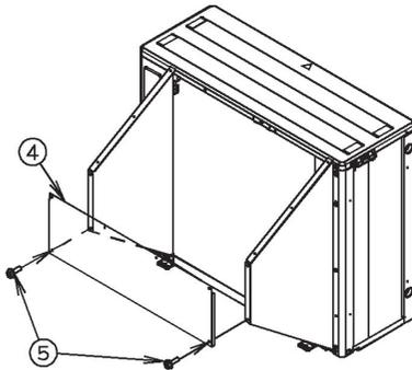
1. Temporarily secure the front plate ④ in place with the 2 screws ⑤ included in the kit.
