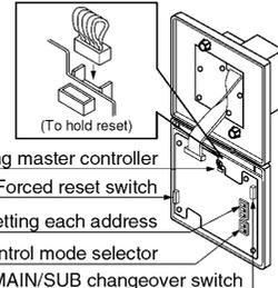
After setting, attach the number seal applicable to respective control range of the attached switch display sticker, as shown in the diagram below.
