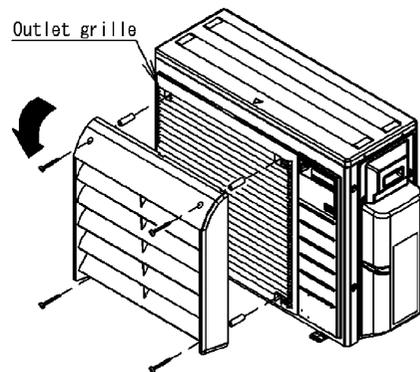
Appearance of the air direction adjustment grille after installation
