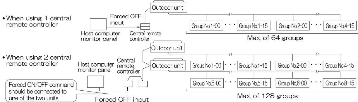
The central remote controller and the separately sold remote control adapter circuit board or group remote control adapter cannot be used together. See the D-BACS design guide for details.
