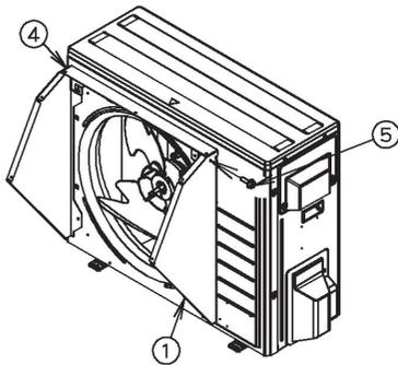
1. Install the side plate (right) ① and installation plate ④ with the 1 screws ⑤ included in the kit.
