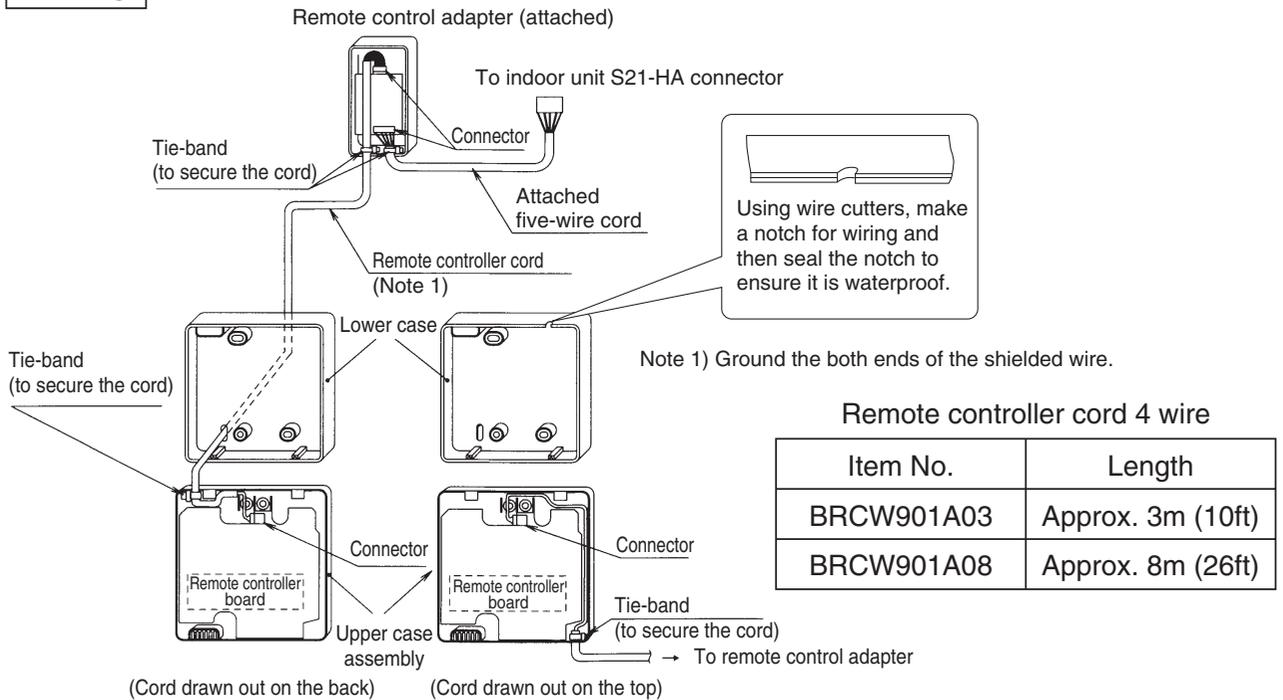
**4. Placing the upper case assembly of the remote controller and the upper case of the remote controller adapter back into their original positions**
