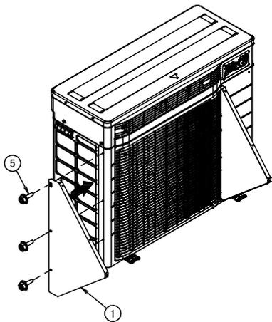
1. Install the side plate (left) (1) on the left side of the front panel of the outdoor unit using 3 screws (4).
