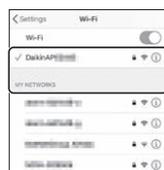
Select the SSID printed on the label attached to the unit or the operation manual, then input the KEY number.
