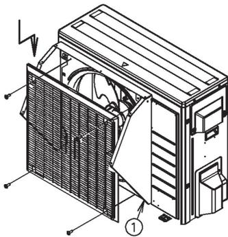
1. When installing the discharge grille removed in [1], jointly tighten the side plate (right) ① with the 2 screws securing the discharge grille. (Secure the discharge grille with the 4 screws and 2 hooks.)
