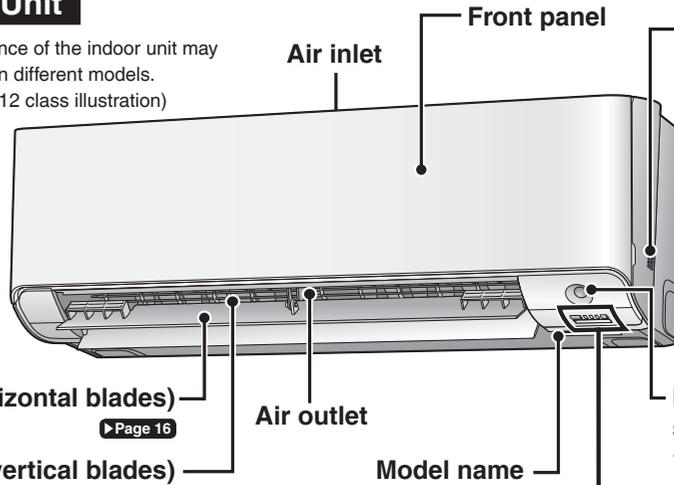
■ **Indoor temperature sensor and Indoor humidity sensor**
