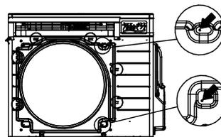
3. After removing the outlet grill, install the side plate (right) (2) using 2 screws (4) at the top and bottom locations indicated by arrows @ in the figure.
