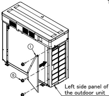
1. Install the side plate (left) (1) on the back of the left side panel of the outdoor unit using 3 screws (5).
