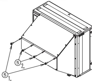
1. Temporarily secure the top plate ③ and front plate ④ to the side plate (right) ① and side plate (left) ② with the 2 screws ⑤ included in the kit.
