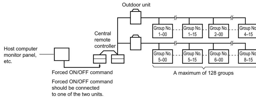
(The central remote controller and the separately sold remote control adapter circuit board or group remote control adapter cannot be used together.)
