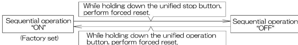
NOTE: The sequential operation function is designed to reduce the load on the power supply equipment, but does not guarantee that compressors will not be started simultaneously. You cannot therefore count on a capacity reduction effect by power supply equipment breaker selection.
