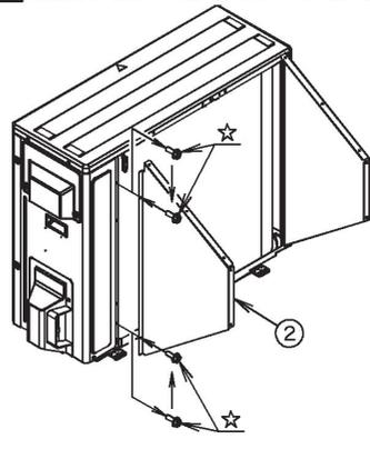
1. Remove the 2 screws (☆) that hold the heat exchanger.
