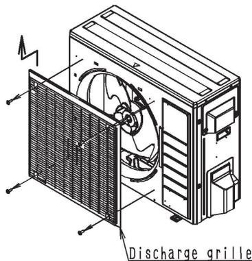
1. Remove the 4 screws that hold the discharge grille. (The discharge grille is held with the 4 screws and 2 hooks.)
