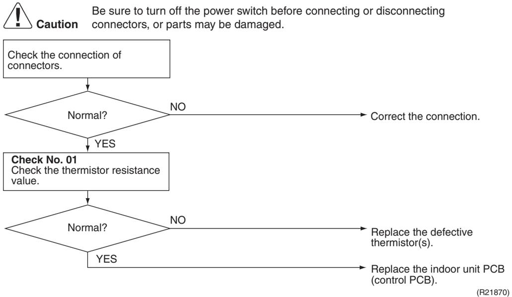
Ⓛ4 : Indoor heat exchanger thermistor
