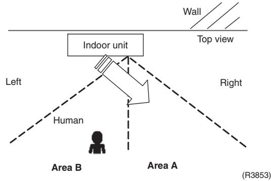
1. Human detection signal ON in both areas A and B: Shift the airflow direction to area B (left side)
