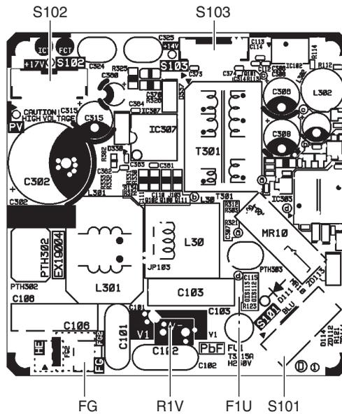
**Display/Signal Receiver PCB (A3P)**
