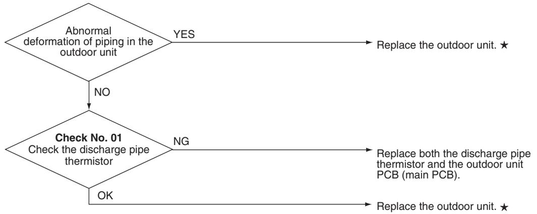
★ Replace the unit as directed in the installation manual, making sure that air does not intrude into the refrigerant piping.
