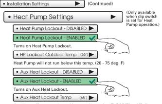
Aux Heat will not run above this temp. (0 - 75 deg. F) GAS/EL or HP dip switch must be set for HP and GAS or ELEC dip switch must be set for ELEC.
