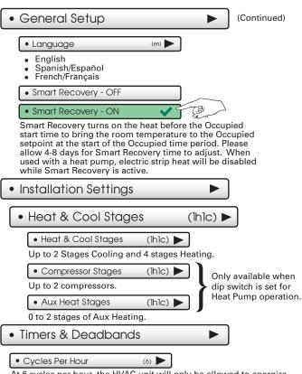
At 6 cycles per hour, the HVAC unit will only be allowed to energize once every 10 minutes. The Cycles Per Hour limit may be overridden and reset by pressing the WARMER or COOLER buttons.
