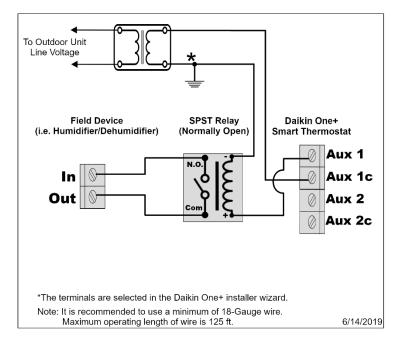
Two accessories can be connected to either pair (Aux 1/1c or Aux 2/2c) of terminals\*.
