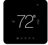
The **home screen** displays the current temperature, the current system mode, and icons leading to each of the top level screens.
