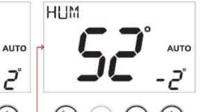
The thermostat humidity will be displayed and may be calibrated using the WARMER (up) and COOLER (down) buttons.
