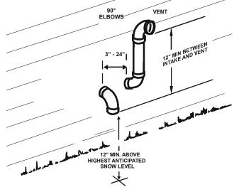
ALTERNATE HORIZONTAL VENT TERMINATION (DUAL PIPE) FIGURE 19
