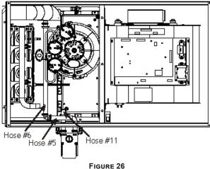
UPFLOW MODEL INSTALLED HORIZONTALLY WITH LEFT SIDE DOWN - ALTERNATE
