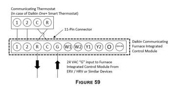
NOTE: PCBKF108 IFC has the added feature of 24 VAC input to G terminal when using a communicating thermostat. ERV/HRV and other accessories can send a signal to the G terminal and energize the continuous fan. The continuous fan speed can be adjusted on switch bank S5, dip switch 3 & 4. The 24 vac source must originate from the R terminal of furnace.
