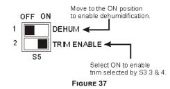
To install/connect a dehumidistat:
