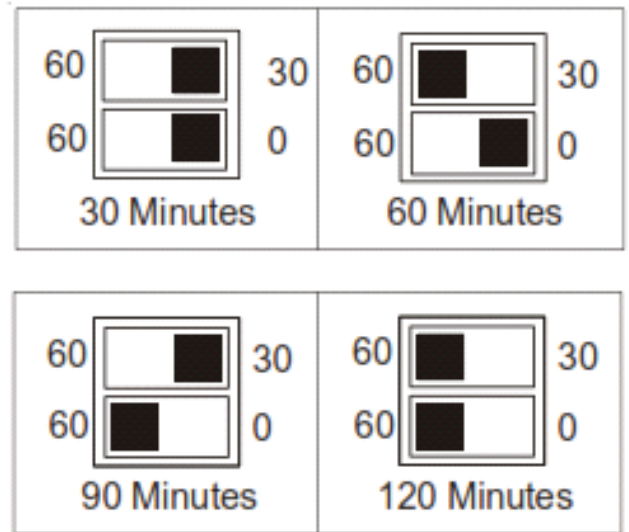
Dipswitch Settings for Selection of Defrost Time
