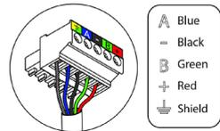
To connect with other DZK system's main boards, use the 2-pin terminal to connect the Webservice Cloud to the automation bus of the other main boards. Use the proper cable: shielded twisted pair 2 wired: 2x0.22 mm<sup>2</sup> (23 AWG – 2 wired). Attach the wires with the terminal screws following the color code.
