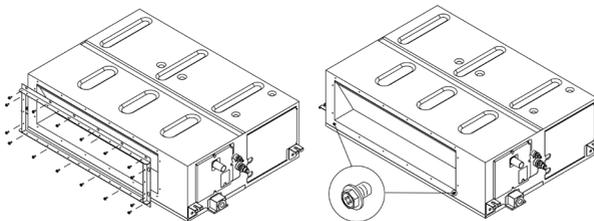
4. Sit the zoning box on the screws as shown below, and then affix the box using the remaining screws.
