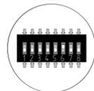
Select other control outputs associated to the zone if necessary. The zone address will be the one with the lowest number selected (for example, associated output 6 to the zone address 5).
