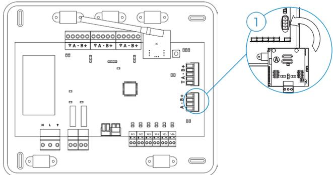
**Error 10: Communication error between the Webserver HUB / BACnet Gateway and the DZK Control Board**
