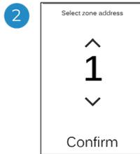
Select the zone associated to this thermostat. Each zone has a corresponding control output.
