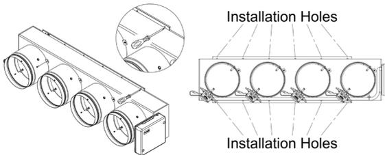
3. Remove the indoor unit collar. Insert a screw (not fully tightened) in the bottom corners of the indoor unit as shown in the following figure:
