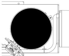
**Keep in mind:** when one or more dampers are disabled, it is recommended to adjust the Airflow control parameter to avoid overpressure on the active dampers and ductwork.
