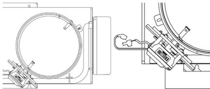
**Keep in mind:** to maximize the air flow for each damper, the best way to disable dampers is to start disabling from the ends to the center, due to the position of the DZK related to the air handler.
