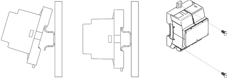
**Note:** To remove the module on DIN rail, pull the the tab down to release it.
