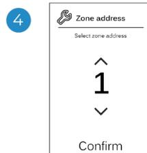
Select the zone associated to this thermostat. Each zone has a corresponding control output (actuator output or radiant element control relay output).
