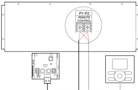
**Important:** The navigation controller can be removed after commissioning the indoor unit as it is not required for the DZK-4 operation.
