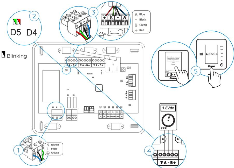
**Error 1: Thermostat (wireless) - Communication error with the DZK Control Board**
