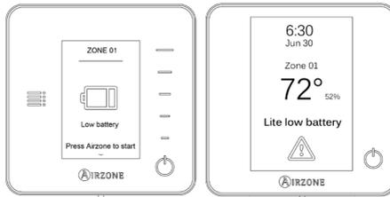
To replace the battery, separate the thermostat from its support and replace the battery (CR2450). Remember to deposit the old battery into an appropriate recycling point.
