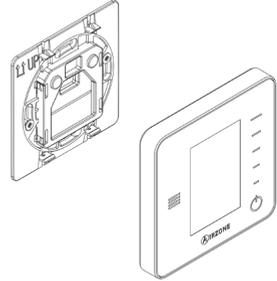
**Important:** perform the pairing of thermostat in their final location. Distances less than 18 inches between the thermostat and the control board can saturate the receivers and make the pairing impossible.
