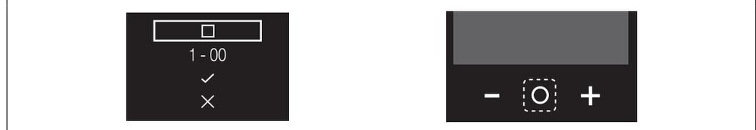
8. Press the **[+]** button to put a check **[✓]** in the box. (It is now possible to edit the DIII-NET group address.)
