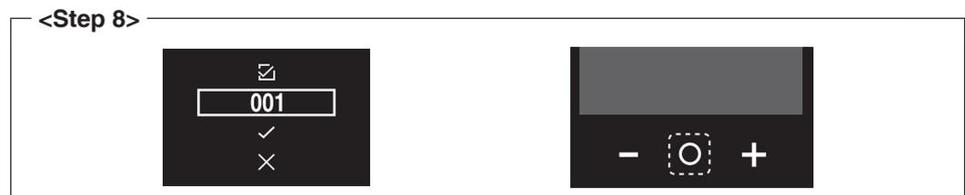
9. Using the **-** and **+** buttons, change the Airnet address.
