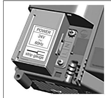
When stripping the wire, be careful not to scratch the finish of the exposed part of the wire.
