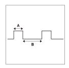
A. Pulse width: 20 to 400 msB. Pulse interval: 100 ms or more
