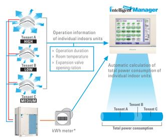
\* Pulse power meter that provides an output of 1 pulse per 1 kw and has a width of 40-400 milliseconds.
