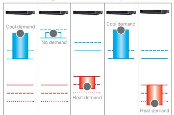
» Option available for heating override if there is an indoor unit which the heating demand exceeds  $(H_SP - (PCd + SCd))$
