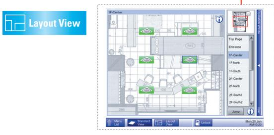
**[Layout view]** A special feature utilizes building floor plans to provide a visual representation of system equipment. The users can visually locate any installed equipment on the floor plan without having to memorize equipment names.
