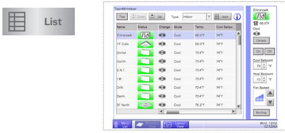
**[List view]** Designed for simplicity, List View provides a quick view of overall status and essential information in a list format. Using the sorting function, the indoor units operating under the same conditions and status are identified for comparison and assessment.
