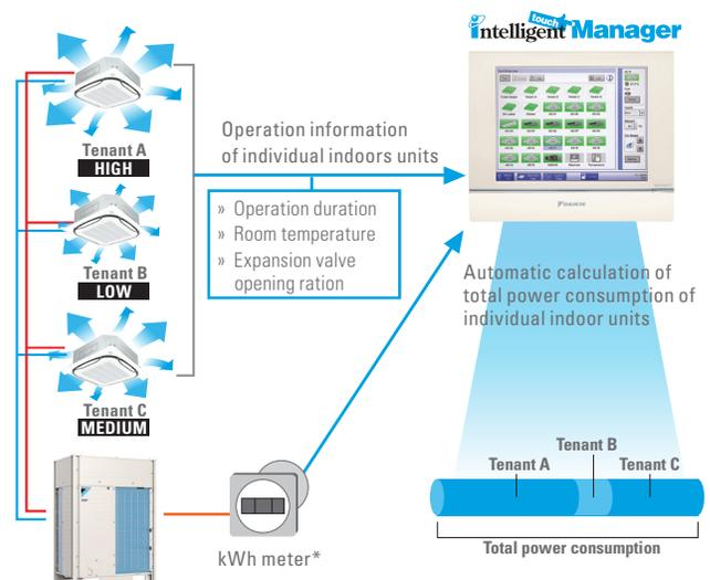
\* Pulse power meter that provides an output of 1 pulse per 1 kw and has a width of 40-400 milliseconds.
