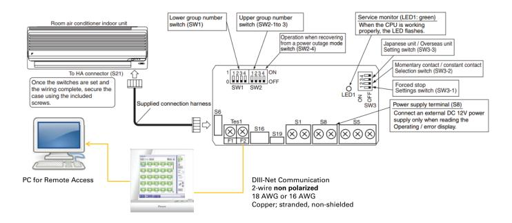
Once the KRP928BB2S is installed, the F1-F2 is wired to the *iTM* or an Interface to allow BMS control. The below table provides the details of the functionality available from each interface using the KRP928BB2S.
