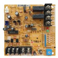
The adaptor offers a few more control features outside of the BMS control. It is important to review the installation manual to select the correct setting. The Single-zone, Multi-zone, and *SkyAir* systems can be integrated in to the Building Management System (BMS) by using a Daikin BACnet<sup>™</sup> BMS Interface or using a dry contact adaptor. Single-zone or *SkyAir* systems are commonly used for cooling IT and equipment rooms on projects that use *VRV* for comfort cooling and heating.
