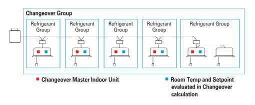
**Vote Method:** This method enables the *iTM* to determine the operation mode by calculating the average room temperatures and the average setpoints of all indoor units in the changeover group. A weight (0-3) can be added to each indoor unit in the changeover group. It is used in cases where there is a desire to evaluate temperature throughout a large physical space, for example when multiple indoor units are installed in hallways.
