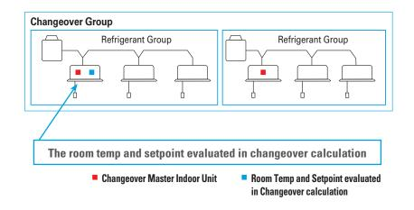
**Individual Method:** This method enables switching between the cooling and heating modes individually for each indoor unit in the changeover group. This method should be used for Heat Recovery systems where each refrigerant group has control of the operation mode without depending on another refrigerant group. For example, in a hotel or nursing home where there are many refrigerant groups, which can be configured with the same changeover configuration.
