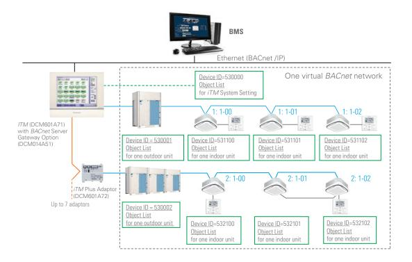
Up to 128 indoor unit and outdoor unit management points can be controlled and monitored through the *iTM BACnet* Server Gateway. The *iTM BACnet* Server software is compatible with the *iTM* Plus Adaptors. The *iTM* Plus Adaptor is intended for use with the *iTM* and shall not be used independently.
