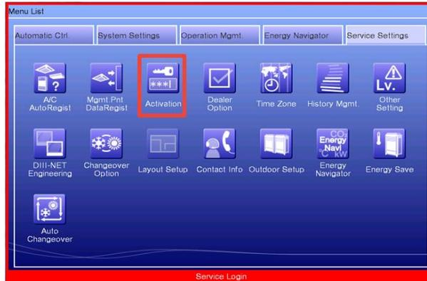
2. On the Activation Setup page, click the Add button to open the keyboard dialog box, and enter the activation key for the *iTM* BACnet Server Gateway option.
