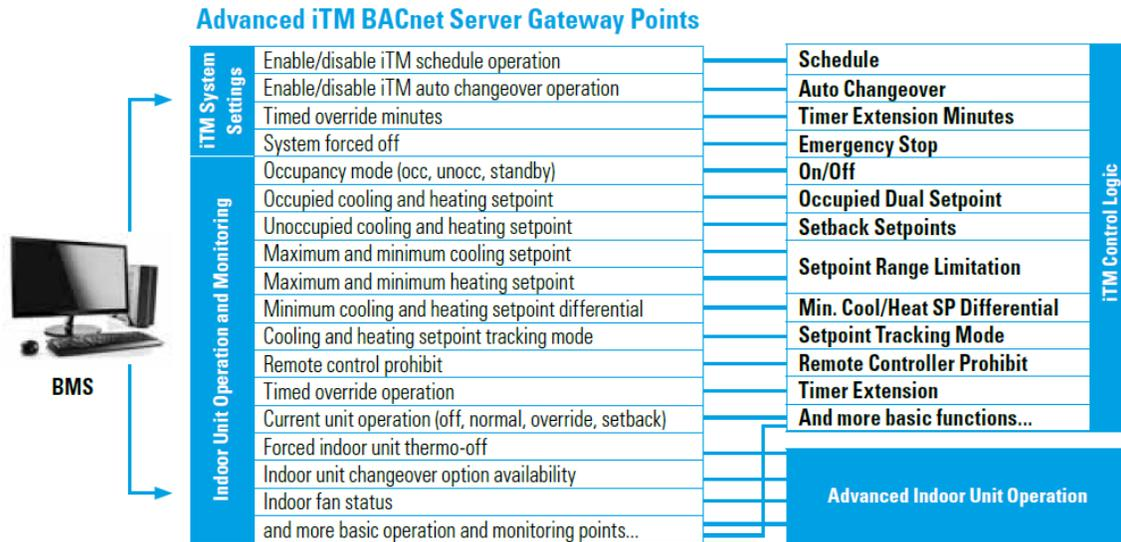
Figure 19. BACnet® Server Gateway Point and *iTM* Logic matchup
