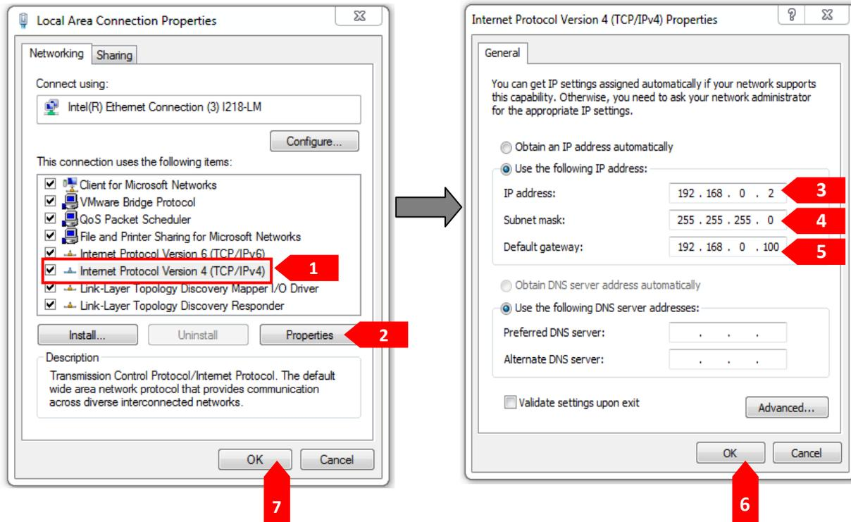
4. Change the test operation PC's IP address.
