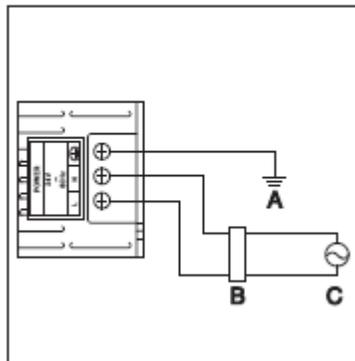
**A.** Earth    **B.** Earth leakage breaker    **C.** Power supply 24VAC 60 Hz
