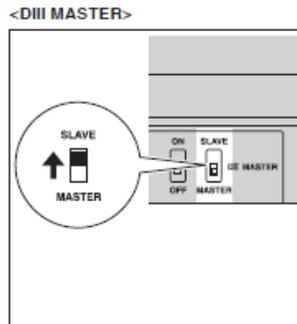
When installing multiple centralized controllers, only set the highest-priority controller to MASTER, and set all other controllers to SLAVE according to the following order of priority.
