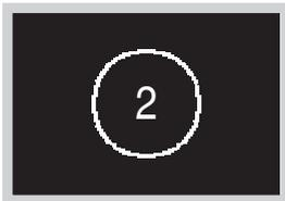
When the U5 error code appears, press
