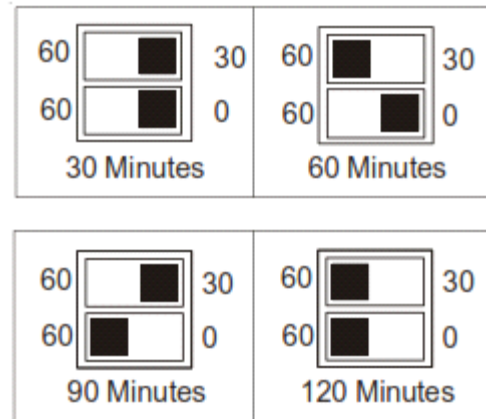
Dipswitch Settings for Selection of Defrost Time
