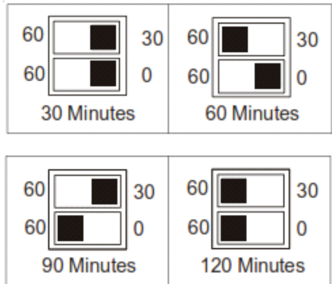
Dipswitch Settings for Selection of Defrost Time
