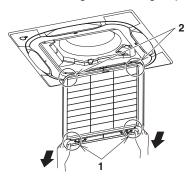
1 Pull the air filter end inclined downward and unhook the hooking hole of the air filter from the projection of the grille. (Both right and left)
