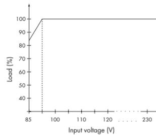
Fig. 6: Input voltage derating curve
