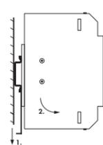
Fig. 2b: Disassembly
