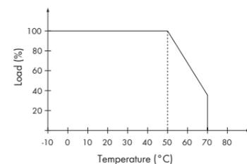
Fig. 5: Temperature derating curve
