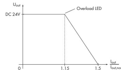
Fig. 4: Output characteristics
